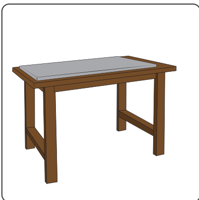
Stable Work Table With Sacrificial Board/Fibre Cement
