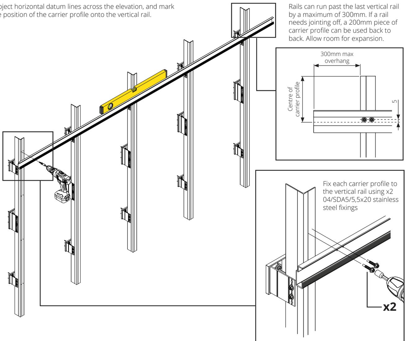
Rails can run past the last vertical rail by a maximum of 300mm. If a rail needs jointing off, a 200mm piece of carrier profile can be used back to back. Allow room for expansion.
