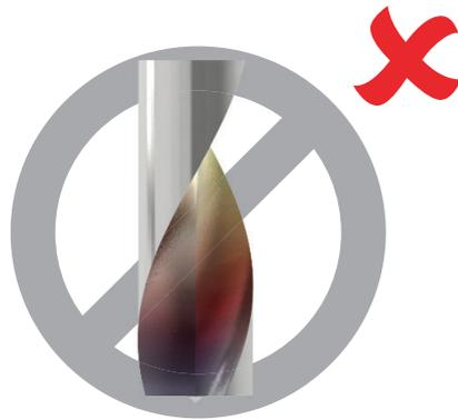
Check for signs of wear. Do not use a worn-out drill bit. Life expectancy for SFS VHM drill bits is approximately 500 holes
