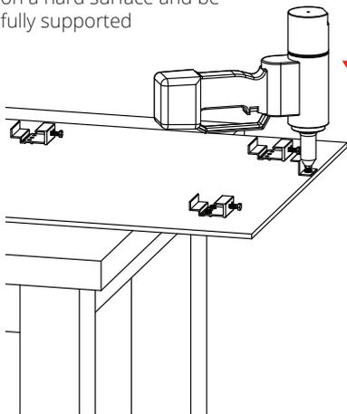
Setting tool must be perpendicular to the panel face
