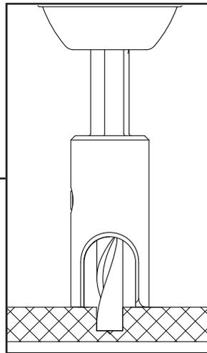
Pre-drill a  $\text{Ø}6\text{mm}$  blind-hole using a milling cutter or a SFS drill bit combined with the SFS universal depth locator.
