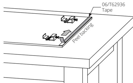
**!** Due to immediate bonding, repositioning the tape is not recommended. Removing the tape from the part is only possible shortly after tape has been applied. Once removed, it cannot be used again and should be discarded.
