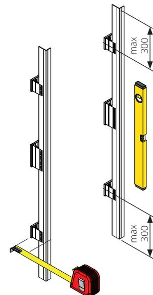
Check and adjust extrusions are in the correct position
