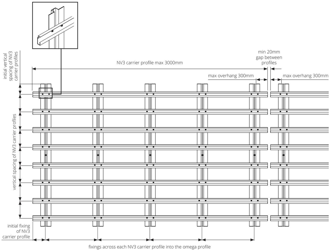
**1** Start with Nvelope NV3 rail system installed and ready to receive cladding panel.
