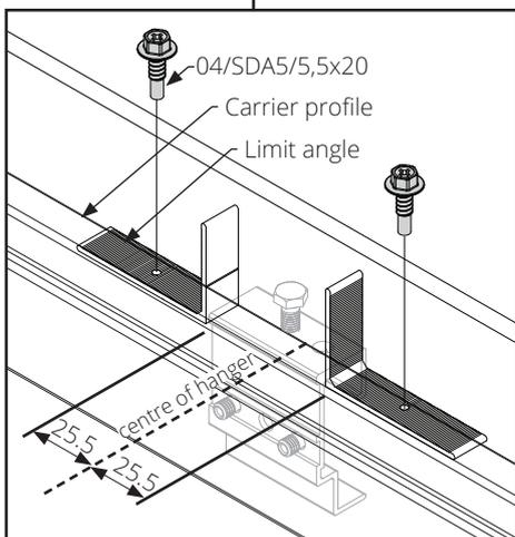
Provides overall 1mm clearance for the hanger
