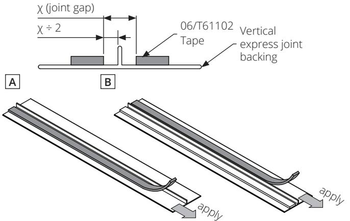
**3** Position vertical express joint backing on the rail. Pre-drill holes for riveting and fix to carrier rail
