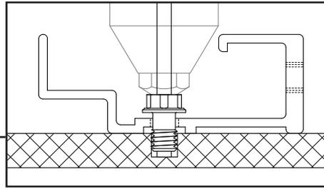
Position the pre-drilled NV3 TUF-S hanger over the hole in the panel and insert the TUF-S anchor.
