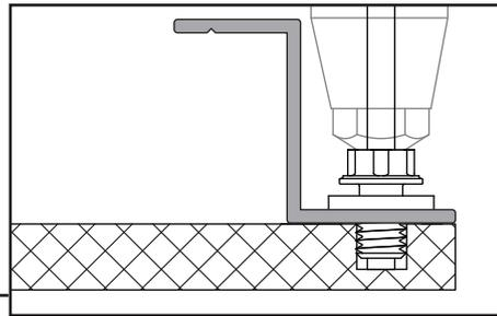
Position the pre-drilled Top slab/ soffit fix clip with the washer over the hole in the panel and insert the TUF-S anchor.
