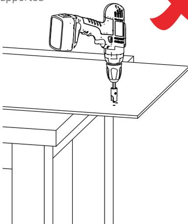
Drill must be held perpendicular to the panel face
