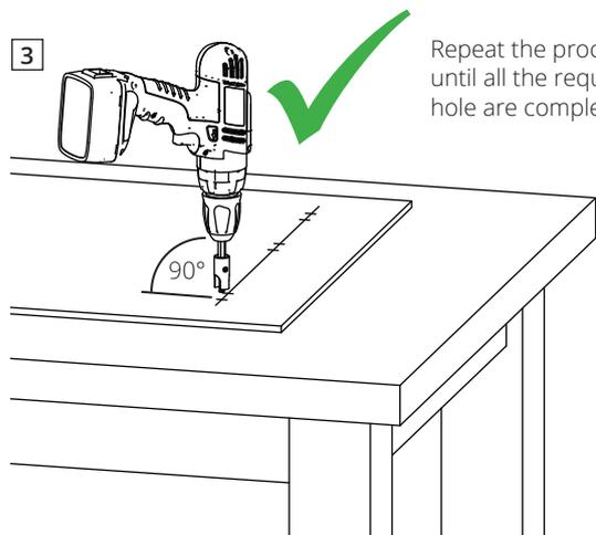
Repeat the process until all the required hole are completed
