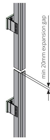
Ensure a 20mm minimum gap between the ends of the rails to allow for expansion. These joints shall coincide with panel horizontal joint i.e. panel shall not bridge over this gap
