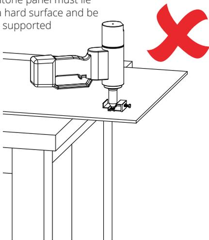
Setting tool must be perpendicular to the panel face
