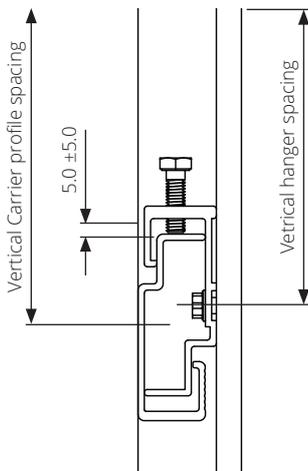
Initial setting of the panel is 5mm from the NV3 carrier profile. Allows for adjustability of  $\pm 5\text{mm}$
