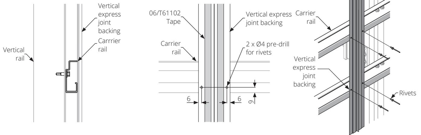
**3 A** Joining vertical express joint backing trims over 3100mm
