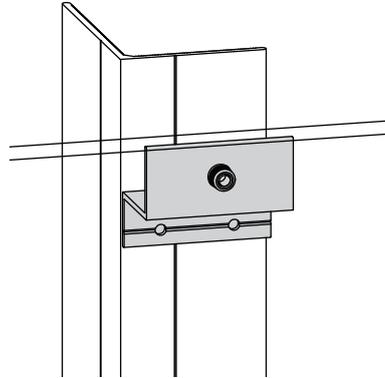
b Rotate clip to align to the vertical rail
