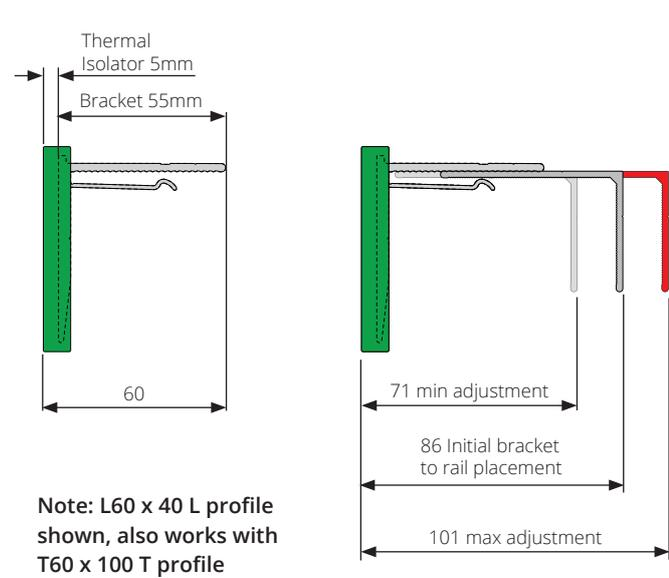
Isolators are included as standard. If isolators are not required, reduce dimensions by 5mm
