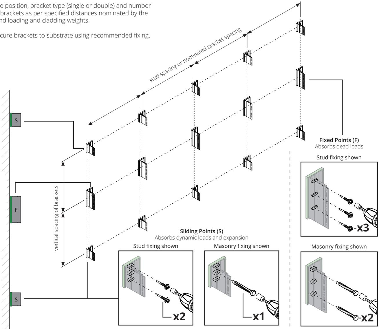
Refer to bracket fixing guide (page 6) for fixing according to the building substrate
