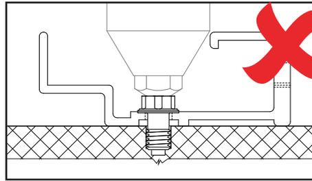
Do not apply force to the TUF-S before setting as this may cause damage to the Equitone panel face
