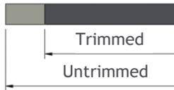
**The panel must not be installed with untrimmed edges.** Approximately 15 mm needs to be trimmed from each of the untrimmed (raw) edges.
