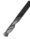
EQUITONE 7 mm drill bit for fixing panels to timber framing, or 11 mm drill bit for fixing panels to metal framing
