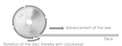
Do an initial test with any new machine or blade on a waste piece of material.
