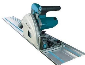
We recommend a fibre cement blade with a cutting speed of 4000-6000 RPM with an external disc diameter of  $\varnothing 160$  mm.
