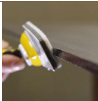
Starting at one side of the panel, angle the applicator away from the face of the panel. Simply run the applicator along the edge. Ensure full coverage of the edge. Repeat the process if necessary.
