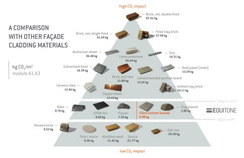
The Construction Material Pyramid was developed by the Centre for Industrialised Architecture [CINARK] at the Royal Danish Academy in 2019. It is a way of visualising the carbon emissions associated with the production of different materials. The pyramid focuses on the product stage [life cycle phases A1 - A3]. It gives an impression of the global warming potential of fibre-cement boards in general compared to other cladding materials.
