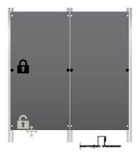
EQUITONE may be face fixed to metal supporting frame using the EQUITONE UNI-rivet. The UNI-rivets have colour matched heads to blend in with the panel. Aluminium UNI-rivets can only be used with aluminium supporting frame. Stainless steel UNI-rivets can be used with, aluminium, galvanised or stainless steel supporting frames.
