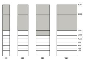
The shaded areas indicate the most uneconomic modules cut from a standard sheet (based on 1220 x 3050 sheet).
