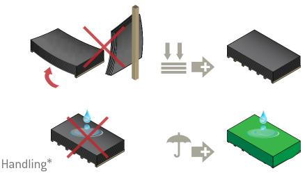
Always lift panels off each other, never slide them over one another, since scratching may occur. To carry the panels, stand them on their back edge and lift with a minimum of two people (one person at each end) protecting the face from scratching or damage. Always lean panel towards back edge to avoid damaging visible front edge. Using soft bearers can help to rest the panel edge on.
