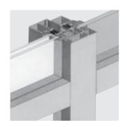
Panelised curtain walling comprises of large prefabricated panels normally a storey height and a bay wide which connect back to the primary structural columns or the floor slab. EQUITONE panels can be used as infill panels in this type of frame. Consultation with the curtain wall supplier is needed to agree the details.
