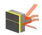
The Ventilated Facade system is very efficient in controlling condensation. Any risk of interstitial condensation occurs in the ventilated cavity. The breathable structure allows water vapour to pass from the inside into the ventilated cavity.
