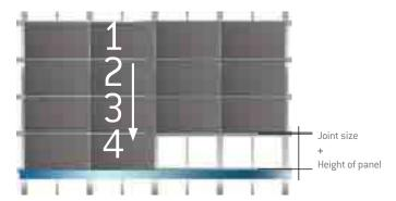
The facade scaffolding can also be stripped down as the cladding proceeds. This ensures no future damage will occur from other trades.
