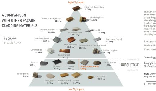
The Construction Material Pyramid was developed by the Centre for Industrialised Architecture (CINARK) at the Royal Danish Academy in 2019. It is a way of visualising the carbon emissions associated with the production of different materials. The pyramid focuses on the product stage (life cycle phases A1 - A3). It gives an impression of the global warming potential of fibre-cement boards in general compared to other cladding materials.
