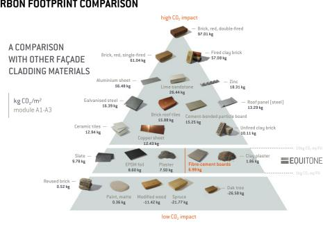
The Construction Material Pyramid was developed by the Centre for Industrialised Architecture (CINARK) at the Royal Danish Academy in 2019. It is a way of visualising the carbon emissions associated with the production of different materials. The pyramid focuses on the product stage (life cycle phases A1 - A3). It gives an impression of the global warming potential of fibre-cement boards in general compared to other cladding materials.
