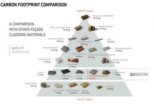
The Construction Material Pyramid was developed by the Centre for Industrialised Architecture [CINARK] at the Royal Danish Academy in 2019. It is a way of visualising the carbon emissions associated with the production of different materials. The pyramid focuses on the product stage (life cycle phases A1 - A3). It gives an impression of the global warming potential of fibre-cement boards in general compared to other cladding materials.
