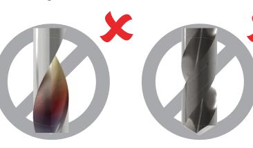
Check for signs of wear. Do not use a worn-out drill bit. Life expectancy for SFS VHM drill bits is approximately 500 holes Do not use a drill bit with a point angle. Anchor will not set into the depth required
