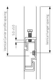
Initial setting of the panel is 5mm from the NV3 carrier profile. Allows for adjustability of ±5mm
