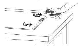
Apply 18 x 1.6 double sided foam tape to the Equitone panel 3 as soon as possible after cleaning to avoid contaminants. Apply pressure to avoid air bubbles under the tape.
