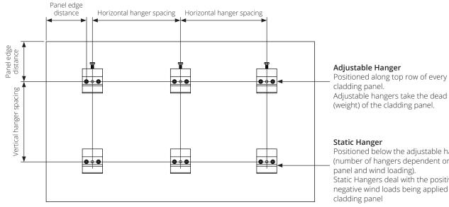
Adjustable hangers take the dead load (weight) of the cladding panel.
