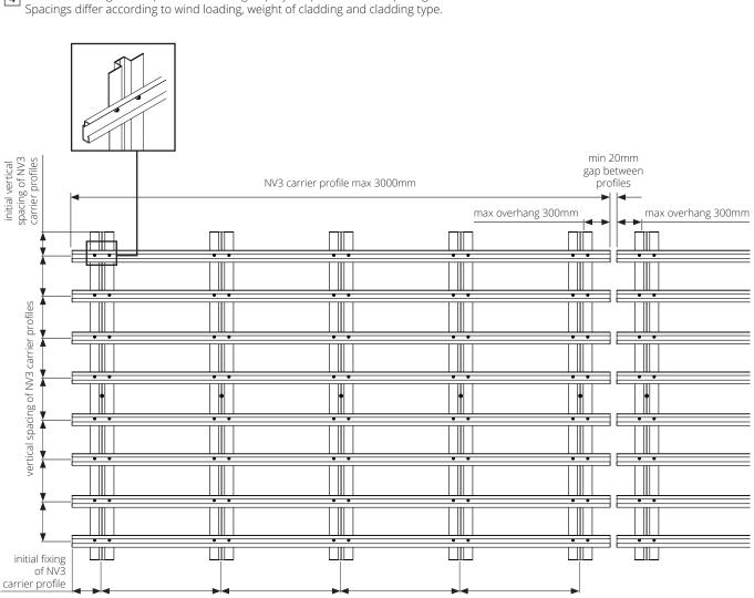
**4** Install remaining carrier profiles according to project specific vertical spacings. Spacings differ according to wind loading, weight of cladding and cladding type.
