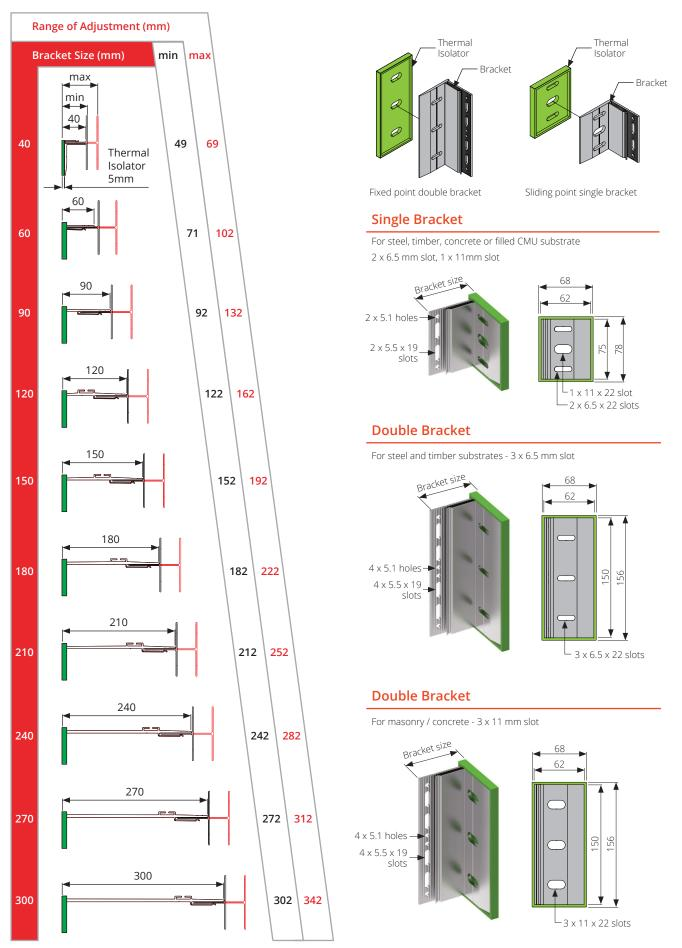
Isolators are included as standard. If isolators are not required, reduce dimensions by 5mm
