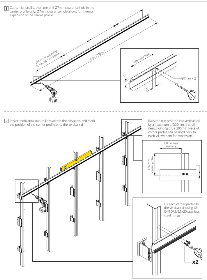
**3** Install remaining carrier profiles according to project specific vertical spacings. Spacings differ according to wind loading, weight of cladding and cladding type.
