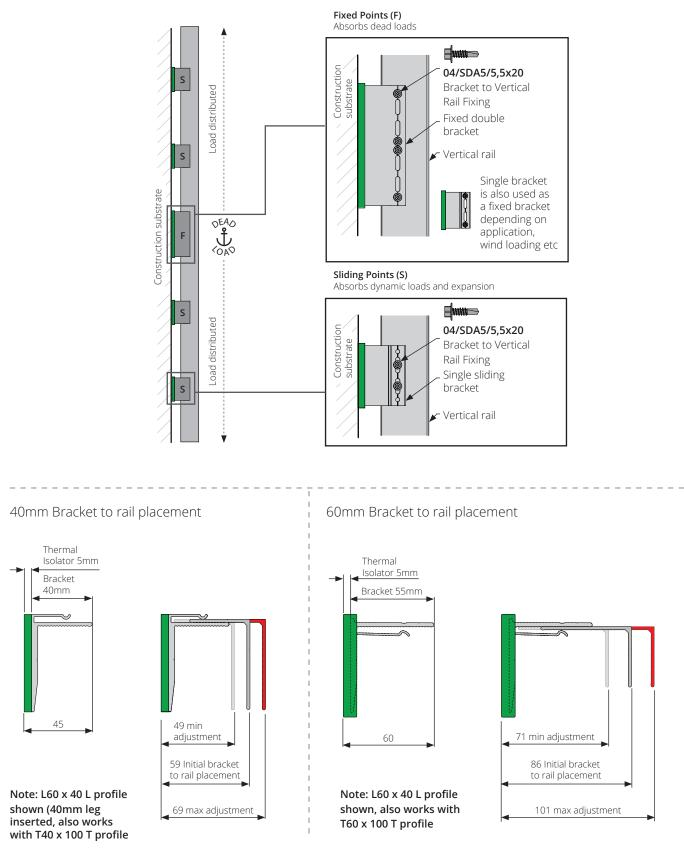
Isolators are included as standard. If isolators are not required, reduce dimensions by 5mm
