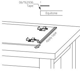
Due to immediate bonding, repositioning the tape is not recommended. Removing the tape from the part is only possible shortly after tape has been applied. Once removed, it cannot be used again and should be discarded.
