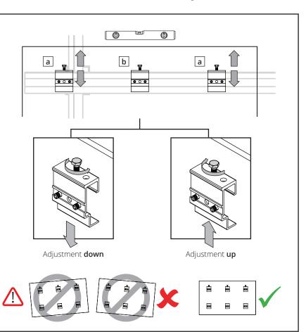
Repeat steps 1 - 4 before fixing the panel for the panels on the same row
