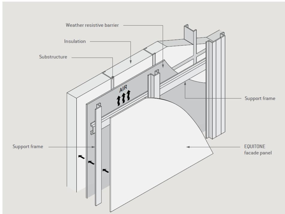
EQUITONE's ventilated façade systems have been independently tested and certified for the purpose of weathertightness compliance in accordance with NCC regulations.
